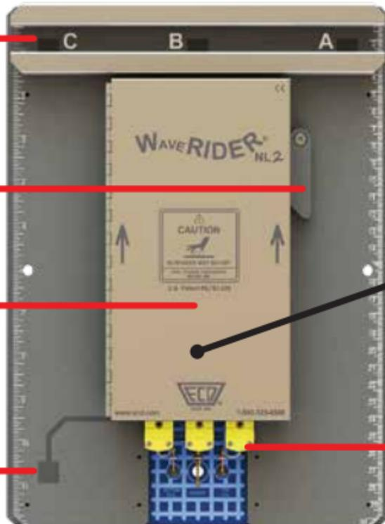
**Extractor handle:** This disconnects the M.O.L.E.<sup>®</sup> Profiler from the connector
