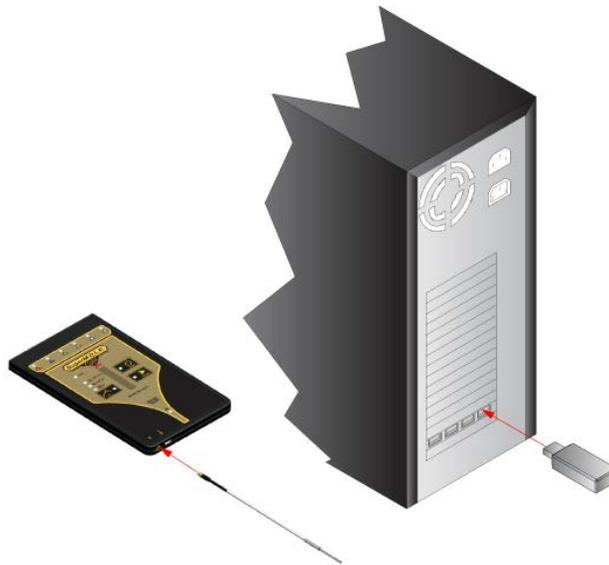
The Transceiver can either be connected directly to a computer USB Port or a USB extension cable. Using a USB extension cable can be a simple way to get the Transceiver to a better reception area without moving the PC. No matter which method is used, keep wires and other metal objects away from the Transceiver.
