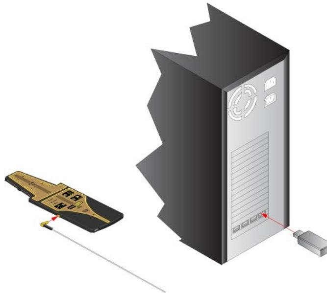
The Transceiver can either be connected directly to a computer USB Port or a USB extension cable. Using an USB extension cable can be a simple way to get the Transceiver to a better reception area without moving the PC. No matter which method is used, keep wires and other metal objects away from the Transceiver.
