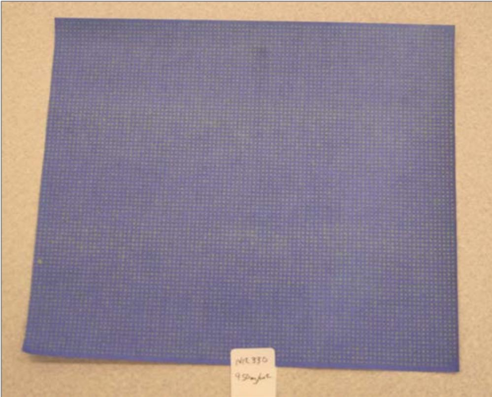
*Figure 6 – Flux Deposition target 950 mg/in<sup>2</sup> using Fluxometer. Very good hole-fill and uniform flux deposition*
