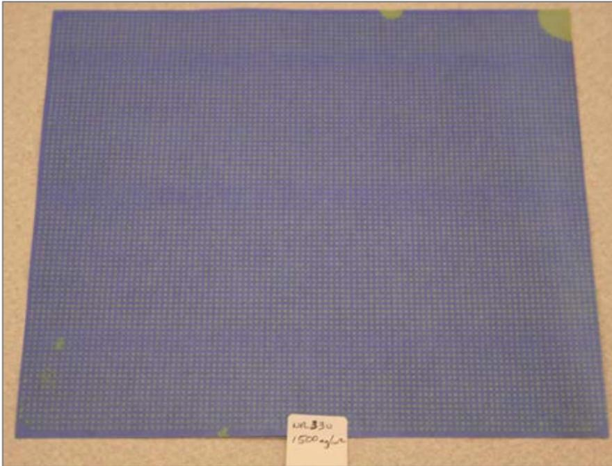
*Figure 8 – Flux deposition 1,500mg/in<sup>2</sup> using Fluxometer Very good hole-fill and uniform flux deposition*
