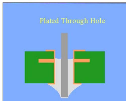
*Figure 9 The solder wets the leads but fails to wet the surface of the through hole.*
