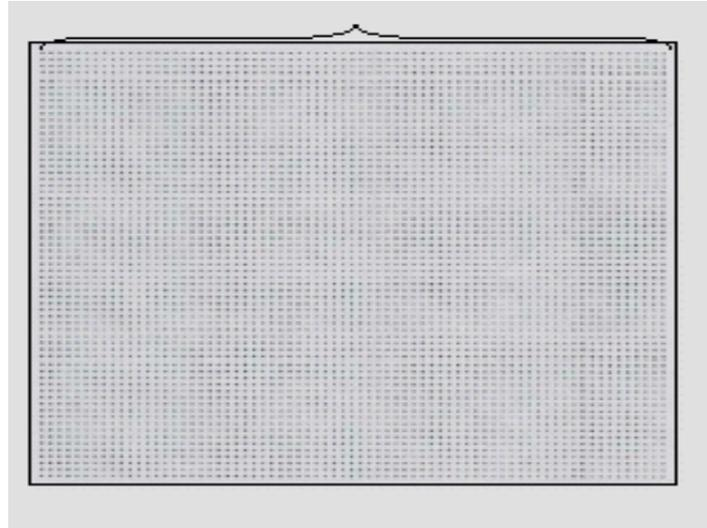
*Figure 15 - Good flux penetration and uniform coverage, all holes are fill and flux penetrated through the mesh/holes*
