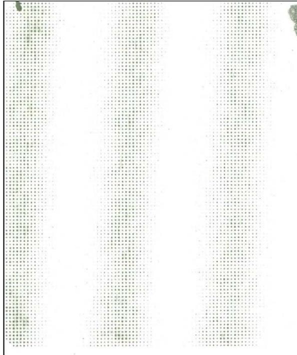
*Figure 20 -Missing spray coverage – no spray on return stroke. Light deposit and hole fill.*
