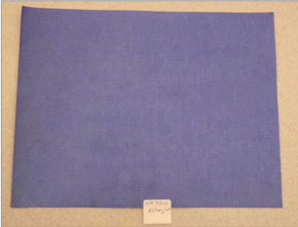
*Figure 4 – Spray deposit target 450 mg/in<sup>2</sup> using Fluxometer. Very good hole-fill and uniform flux deposition*
