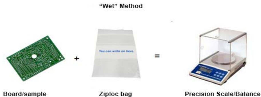
*Figure 1 – Tools required to measure flux deposition on a board in wet method*
