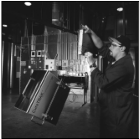
Product profiling in process using ECD CureTRAK™.
